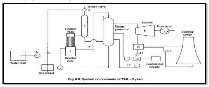
The demineraliser (12) contains resin beads to clean condensate. A problem in the demineraliser arose and this led to the closure of the outlet valve of (12) to the steam generator (3). This resulted in shut down of main feed water pump (13) and the auxiliary feed water pump (14) failed.
